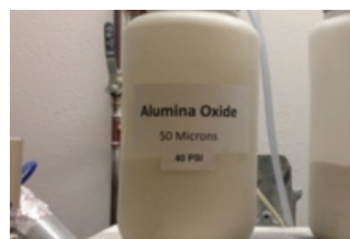
Aluminum Oxide Used to Clean Inside Restoration
